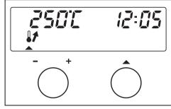
■ Whilst the triangle ▲ is flashing underneath the 17 symbol, use the (-/+) input dial to set the temperature to its highest setting (250 °C).
